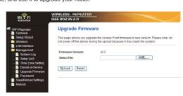
After a firmware upgrade file is selected, click 'Upload' button, and the router will start firmware upgrade procedure automatically. The procedure may take several minutes, please be patient.
